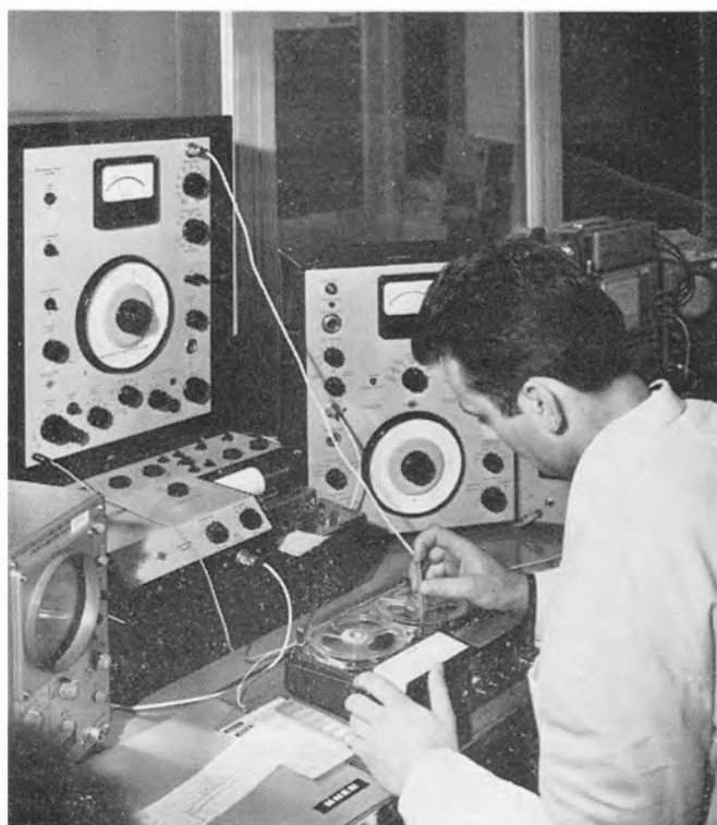
Fig. 2. Every Uher tape recorder is subjected to extensive final testing. Here the frequency response is pen-graphed by B. & K. response testing equipment.
